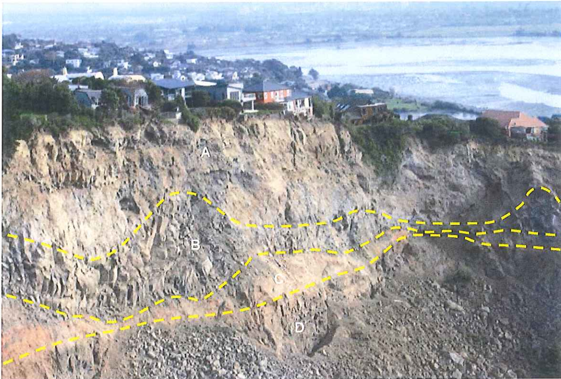
Figure 14 View to the west onto the main cliff at Redcliffs. (A) is basalt lava breccia, (B) is columnar jointed basalt lava and breccia (C) is the epiclastic layer that generally forms a recessive slope, and the material below this is basalt lava breccia (D). Photograph by C. Gibbons (July 2011). For surveyed boundaries between materials refer to Appendix 3.
