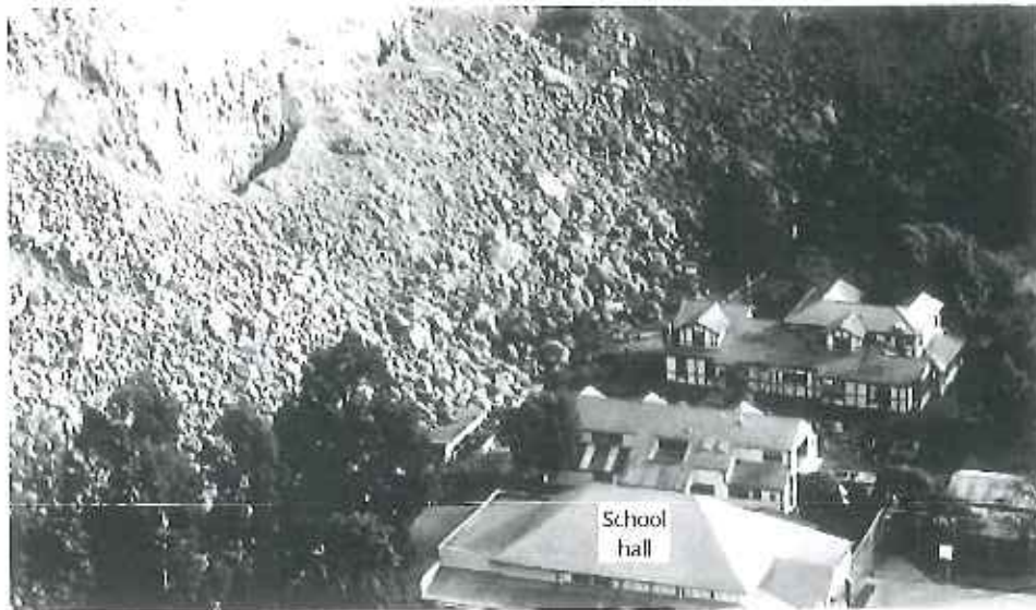
Figure 3: Aerial view of the talus slope below the cliff after the 22 February 2011 earthquake, and before the 13 June 2011 earthquake. Note school hall with reddish roof in foreground. (Source: GNS report 2014/78, Figure 6, August 2014)
